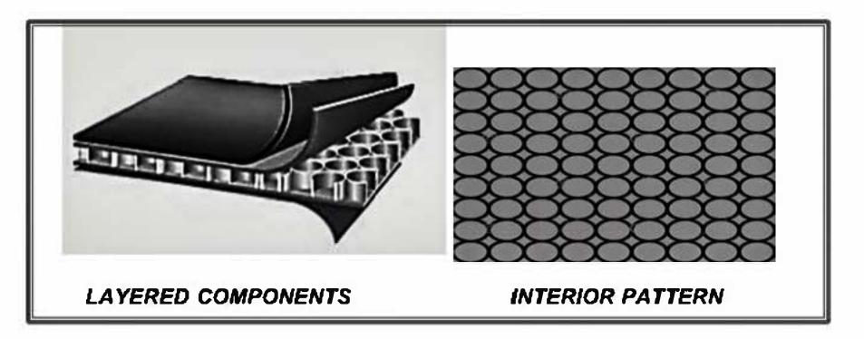
The drawing below illustrates the 8' x 4' sheets innovative design allowing the product to be cut in any direction for adaptability and minmizes waste.
